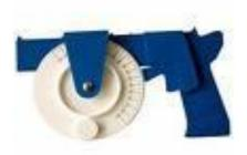
This instrument is generally used to obtain roughly the slope angle of the ground. It consists of a rectangular, telescopic tube (without lenses) about 125mm long with a graduated arc attached. A small bubble is fixed to the vernier arm, once the image of the bubble is seen reflected in the eyepiece the angle of the line of sight can be read off with the aid of the reading glass.
