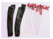
Arrow consists of a piece of steel wire about 0.5m long, and are used for marking temporary stations. A piece of coloured cloth, white or red ribbon is usually attached or tied to the end of the arrow to be clearly seen on the field.
