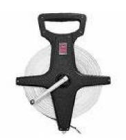
This may be 30m, 50m or 100m long and 13mm wide. It has handles similar to those on the chain and is wound on a steel cross. It is more accurate but less robust than the chain. The operating tension and temperature for which it was graduated should be indicated on the band.
